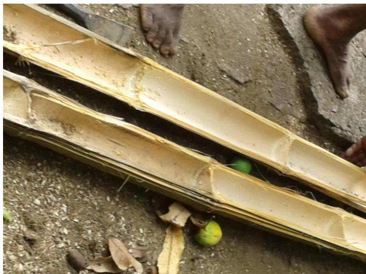
Split lengths of Giant Bamboo with some nodes removed
